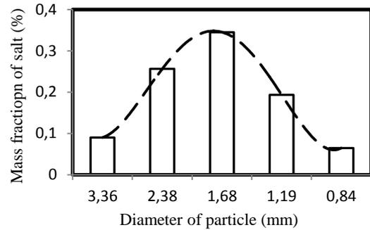
**Figure 1.** Typical size distribution of sample particles.
