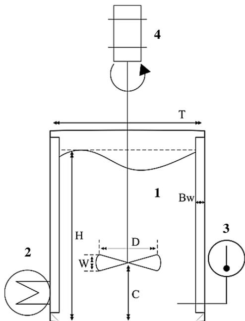
**Figure 2.** Stirred tank used to evaluate the dissolution of a population of salt particles.
